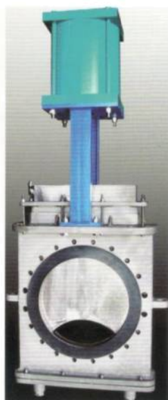
Above: 24" Figure 92 metal seat knife gate for throttling in oil sands. Tungsten carbide overlay on gate face, ID, and port ID.
