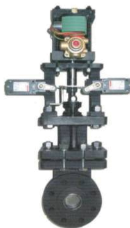
Above: Figure F176 , with air cylinders, open and closed position limit switches, and solenoid control valves. 310 SS for high temperature service.
